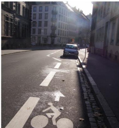
Figure 27: Curbside Bike Lane in Strasbourg
